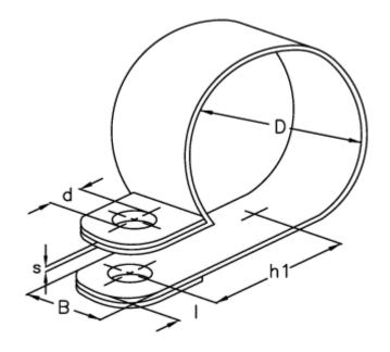
$\begin{array}{ll} d & = 8.4 \\ \mbox{Diameter D} = 62 \\ \mbox{h1} & = 43.5 \\ \mbox{I} & = 8.5 \\ \mbox{s} & = 0.8 \\ \mbox{Width B} & = 20 \\ \end{array}$
